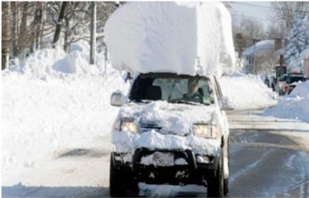
Another area to consider is the vehicle HVAC system. Most vehicles' fresh-air intakes are located just below the front wipers. When loose snow isn't cleared off before starting the vehicle and turning on the heater, this snow can be drawn into the system, where it can waterlog a cabin air filter or cause problems with heater control doors and linkages.
