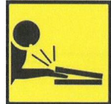
2. Expect the unexpected. When using wrenches and other hand tools, with which you expect resistance, anticipate that the tool might slip or the object to which pressure is being applied may suddenly give way.
